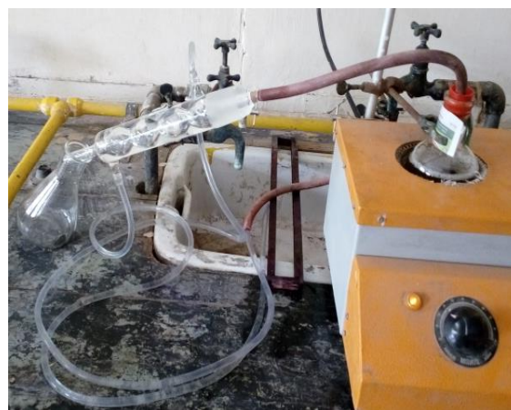
Figure:14 Distillation unit for ethanol recovery
