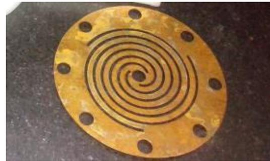
Fig 14 spiral flexure from Be-Cu sheet metal part
