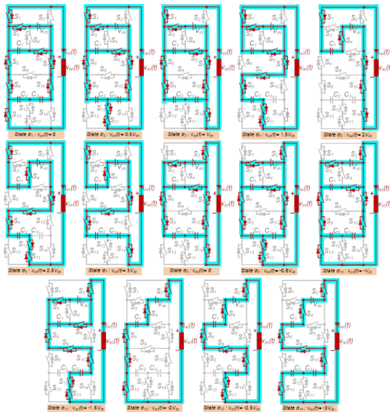
Fig.2. Working states for the proposed thirteen-level inverter with switched capacitors
