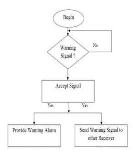
Figure 5: Receiving part work flow
