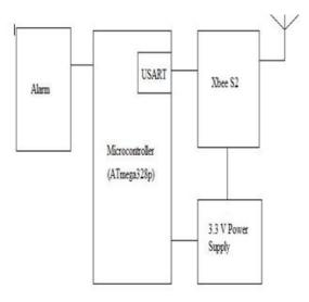
Figure 2: Receiving Part of wireless earthquake
