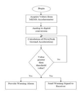
Figure 4: Transmitting part work flow
