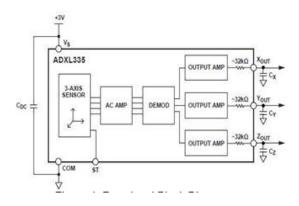
Figure 3: Functional Block Diagram
