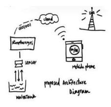
Ultrasonic distance sensors are designed to measure distance between the source and target using ultrasonic waves. HC-SR04 is a commonly used module for non contact distance measurement for distances from 2cm to 400cm. It consists of an ultrasonic transmitter, receiver and control circuit. The transmitter transmits short bursts which gets reflected by target and are picked up by the receiver. The time difference between transmission and reception of ultrasonic signals is calculated.
