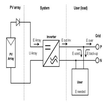
Figure 1. Block Diagram of Grid Connected PV system.
