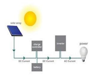
Figure 2. Block Diagram of stand Alone System
