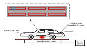
Fig.3: Latest ongoing model for OLEV
