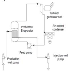
Fig. 2: Example binary-cycle geothermal power plant.
