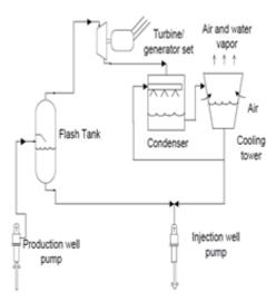
Fig. 1: Example flash-steam geothermal power plant.
