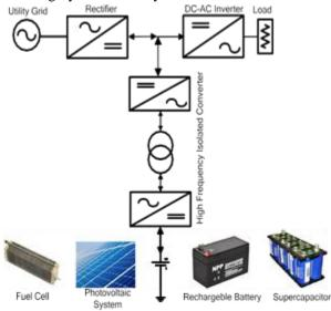
Fig. 4: - Block Diagram of Intelligent UPS system
