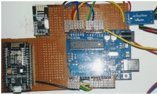
Fig. 5: - Sensing and routing node pcb
