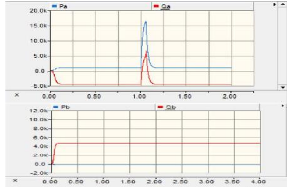
Fig. 10: - Simulation result L-L-L fault on single bus system of both active and reactive power of the generator A
