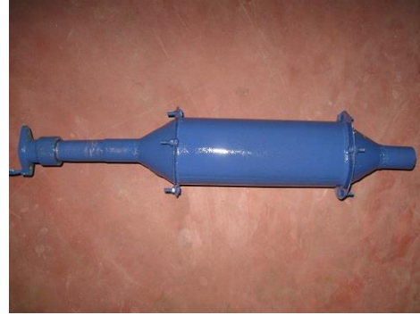
Fig 8: SCR pipe of this project
