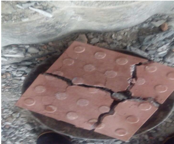
Fig 4.1: Failure of specimen under compression
