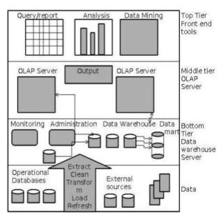
Fig 1: data warehouse three tier architecture
