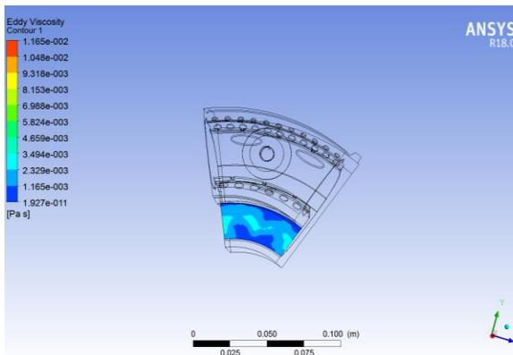
Figure 10: Eddy Viscosity profile at the outlet of the combustor
