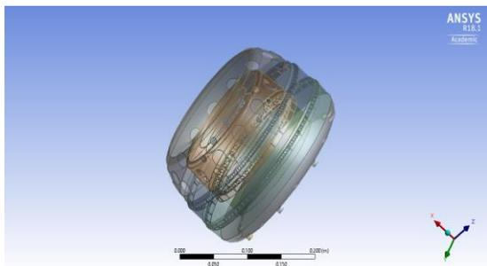
Figure 2: Model of the Reverse Flow Annular Combustor
