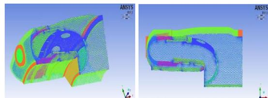
Figure 4: Meshed model of the combustor section
