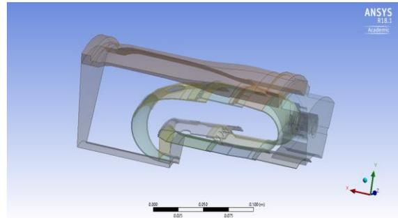
Figure 3: Section of the combustor for simulation
