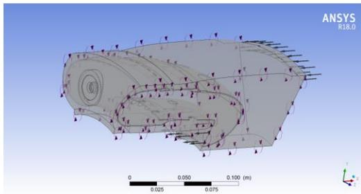
Figure 5: Combustor model with boundary conditions
