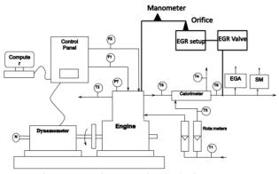
Figure 1. Engine Test-rig block diagram
