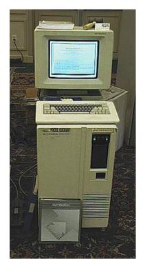
Fig. 2: A Symbolics Lisp Machine: an early platform for expert systems
