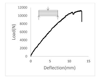
permanent deformation of 5mm of the bamboo (Fig. 3). A good bond integrity was ensured.
