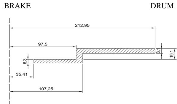
Brake drums must have sufficient strength to resist the mechanical and thermal stresses developed during braking. To satisfy these requirements the drum material should possess a high thermal conductivity, thermal capacity, and low coefficient of thermal
