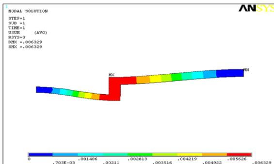
Figure: Thermal deformation for aluminum composite material
