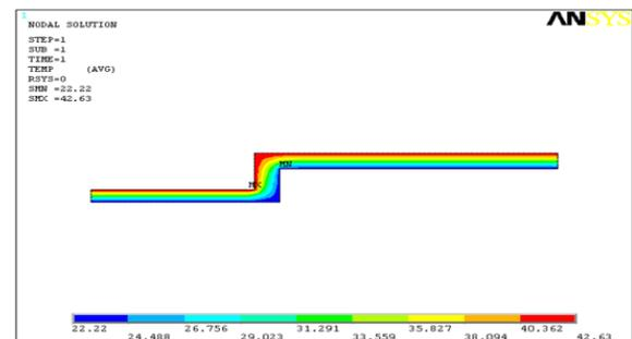
Figure: Temperature distribution for cast iron material in steady state condition
