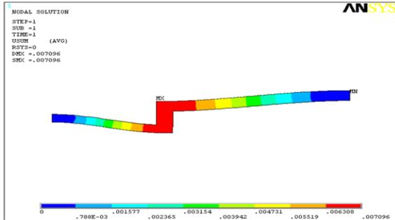
Figure: Thermal deformation for cast iron material
