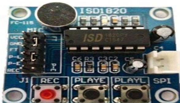
Fig. 3: ISD 1820 voice module
