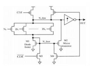
Fig5: Diode flat-footed Domino Logic [2]
