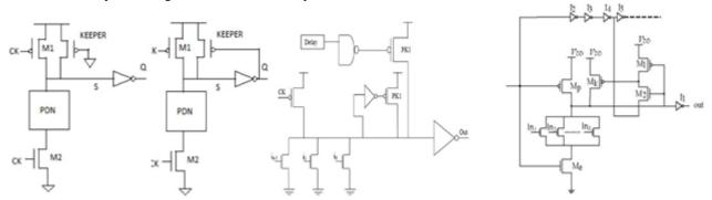
Fig2: Improving noise immunity of dynamic logic gates using (a) Always-on keeper. (b) Feedback keeper. (c) Conditional keeper.(d) Saturated keeper[2]
