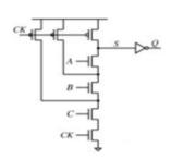
Fig. 4: (a) Precharging all internal nodes[2]
