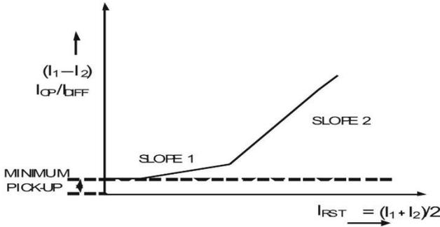
proper sensitivity and security. Knee point of dual slope differential current is decided where saturation of CT is started.
