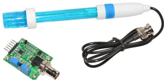
Fig. 2.4: pH sensor with probe
