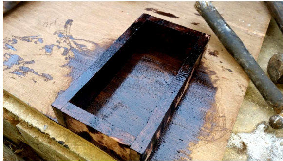
Fig 1. Brick mould of size 190 x 90 x 40mm
