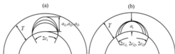
Fig 5. Two sets of initial crack geometries for internal radial-circumferential surface crack (a) when the initial circumference half crack length is fixed; (b) when the initial crack is fixed.
