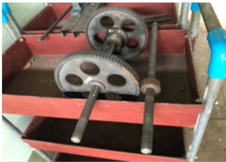
Figure5. (a) Large gear; (b) large gear with sprocket; and (c) assembly of gears
