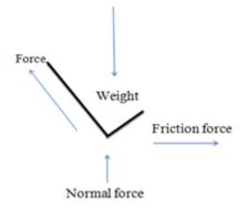
Figure 7. Force acting on the trolley
