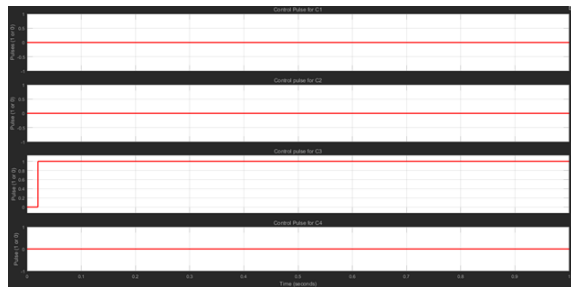
Figure 7: switching pattern of capacitors for PK mill expeller motor section
