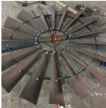
Figure 3. Design of Blade Assembly
