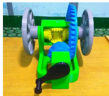
Fig. 1. Differential of Automobile for Teaching Aid
