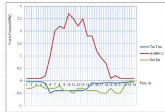
Figure 3. Daily Load Utility Curve of Outgoing Feeders of Ohntaw Substation 66 kV side
