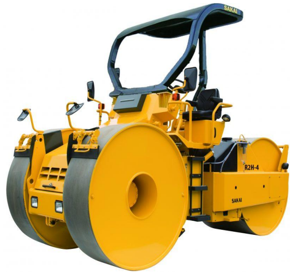
Figure 7. Three-Wheels Roller (Sakai R2H-2K 3)
