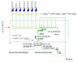
Figure.8 Main Distribution Board Single Line Drawing for Orient Hotel
