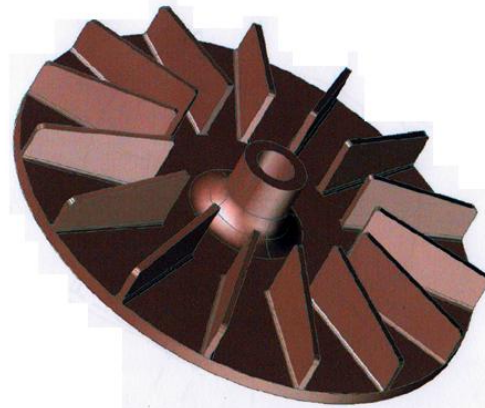
Fig.7. Three-D Model of Radial type Centrifugal Compressor Impeller
