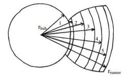
Figure 5. Five sections of the blade
