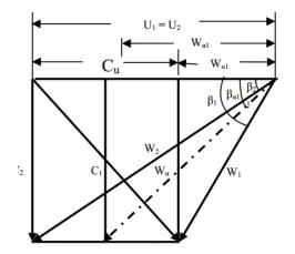
Figure 6. Inlet and Outlet Velocity Triangle
