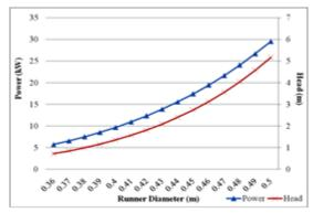
Figure 11. Turbine Performance Curve at Different Runner Diameter for Head and Power at Constant Turbine Speed
