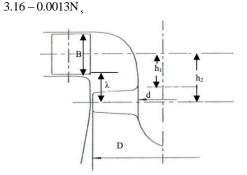
Figure 8. Section View of Propeller Turbine
