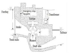
Figure 1 Propeller Turbine [78Ham]
