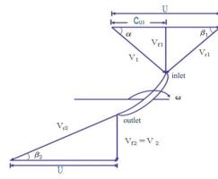
Figure 3. Inlet and outlet velocity diagram of propeller turbine [7]
