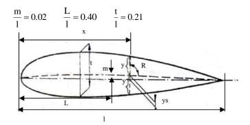
Figure 4. Geometric characteristics of airfoils [6]
