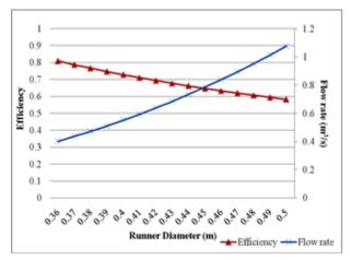
Figure 10. Turbine Performance Curve at Different Runner Diameter for Efficiency and Flow Rate at Constant Turbine Speed
