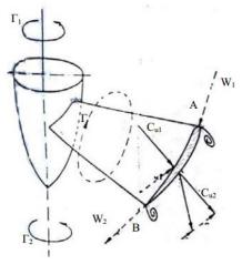
Figure 7. Circularation around the blade
