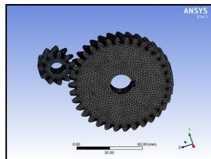
Figure 3. Meshed 3-D model of Helical Gear Pair
