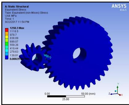
Figure 12. von-Mises Stress of Helix 23° with Stainless Steel
