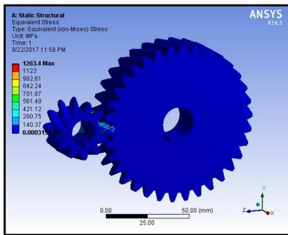
Figure 13. von-Mises Stress of Helix 23° with Structural Steel
