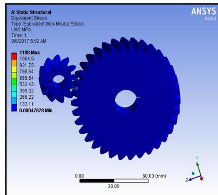
Figure 7. von-Mises Stress of Helix Angle 26° at First Gear Pair
