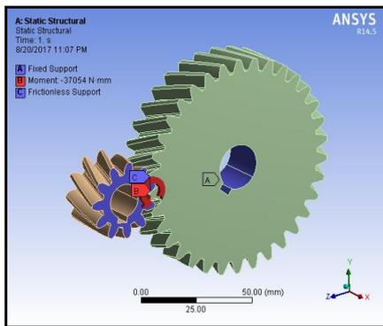
Figure 4. Boundary Condition of Helical Gear Pair
