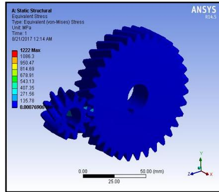
Figure 6. von-Mises Stress of Helix Angle 23° at First Gear Pair
