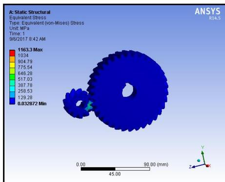
Figure 9. von-Mises Stress of Helix Angle 32° at First Gear Pair
