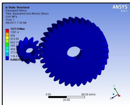
Figure 5. von-Mises Stress of Helix Angle 20° at First Gear Pair
