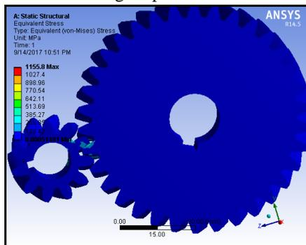
Figure 10. von-Mises Stress of Helix Angle 35° at First Gear Pair
