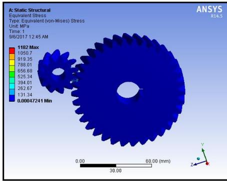
Figure 8. von-Mises Stress of Helix Angle 29° at First Gear Pair
