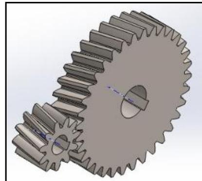
Figure 2. 3D Solid Model of Contact Gear Pair
