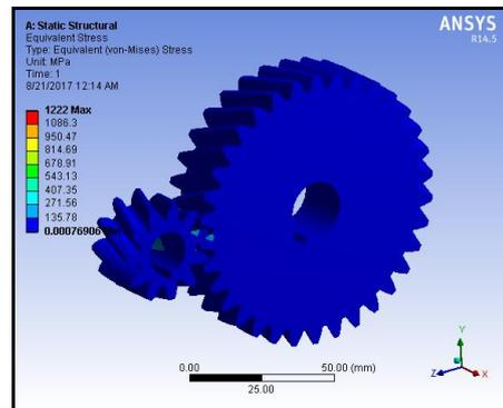
Figure 11. von-Mises Stress for AISI 5160 OQT 400
