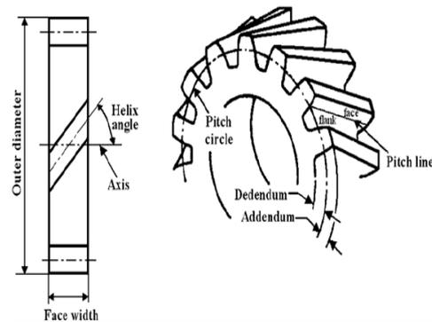
Figure 1: Nomenclature of Helical Gear [4]
