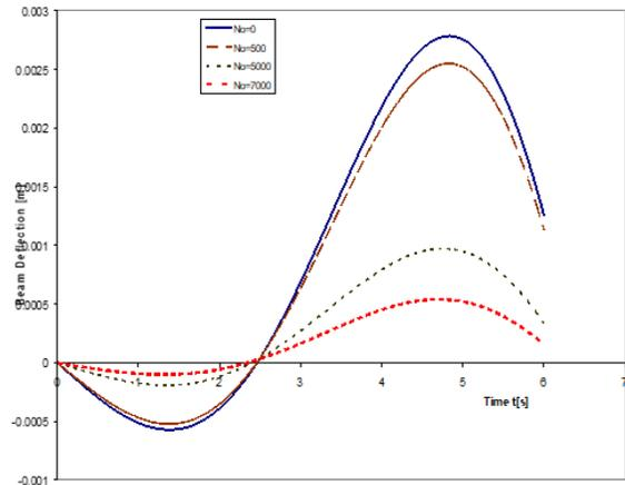
Figure 4: Transverse displacement response of a non-prismatic rotating Timoshenko beam resting on elastic foundation and subjected to Harmonic variable magnitude moving loads for various values of prestress N and for fixed value of foundation modulus
