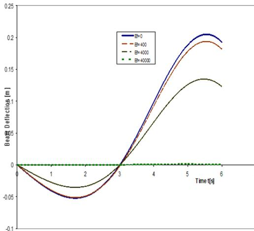
Figure 1: Transverse displacement of a non-prismatic rotating Timoshenko beam under the actions of constant moving force for various values of foundation moduli  $E_f$ .
