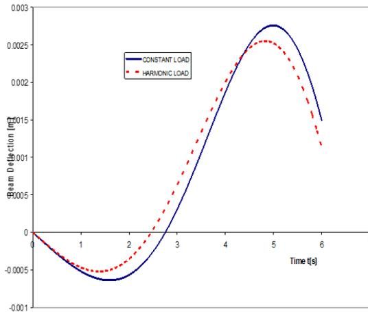
Figure 6: Comparison of the response of the non-prismatic rotating Timoshenko beam to constant and variable magnitude moving load for foundation modulus  $E_f$  and prestress N.
