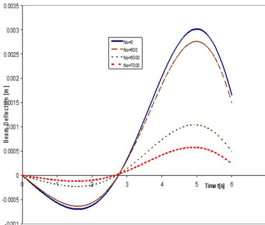
Figure 2: Displacement response of a non-prismatic rotating Timoshenko beam on elastic foundation and traversed by moving constant force for various values of N.
