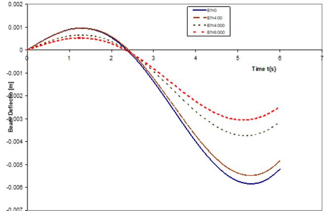
Figure 3: Deflection profile of a non-prismatic rotating Timoshenko beam subjected to Harmonic variable magnitude moving loads for various values of foundation moduli  $E_f$  and for fixed values of prestress N
