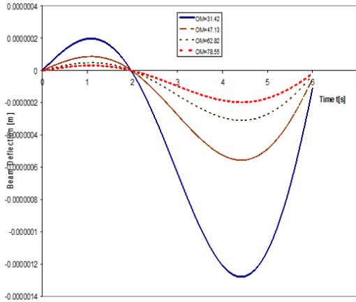
FIGURE 5. The response amplitude of a non-prismatic rotating Timoshenko beam resting on elastic foundation and under the actions of moving load for various values of circular frequency  $\omega$ .
