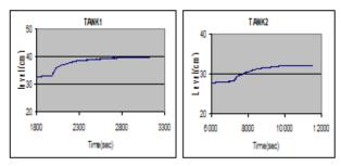
Fig 3. Change in inflow of 10ml /sec given to tank – 1 at 2,000 (sec)
