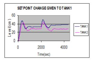
Fig. 7 Servo and regulatory response of Effective transfer function method for a set point change from 33cm to 38cm given at t=2,000 (sec)
