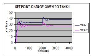
Fig. 5 Servo and regulatory response of Equivalent transfer function method for a set point change from 33cm to 38cm given at t=2,000 (sec)
