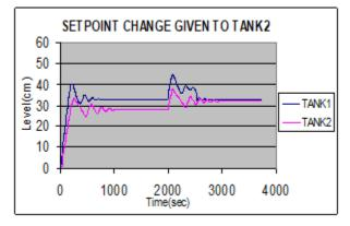
Fig. 6 Servo and regulatory response of Equivalent transfer function method for a set point change from 28cm to 32cm given at t=2,000 (sec)
