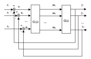
Fig.1 closed-loop multivariable control system
