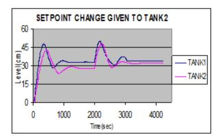
Fig. 8 Servo and regulatory response of Effective transfer function method for a set point change from 28cm to 32cm given at t=2,000 (sec)
