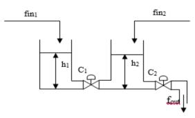
Fig. 2 Two Tank Interacting System
