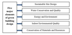
Fig.1: components of green building design (USGBC).
