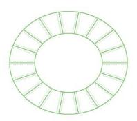
Fig.1 Twenty-Four Slot Stator Geometry
