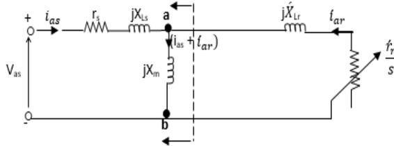
Fig 5: Modified per-phase equivalent circuit of an induction motor at run condition.
