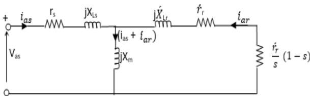
Fig 4: Per phase equivalent circuit of an induction motor which account for copper loss  $(i_{ar})^2 r_r$  in the rotor circuit.
