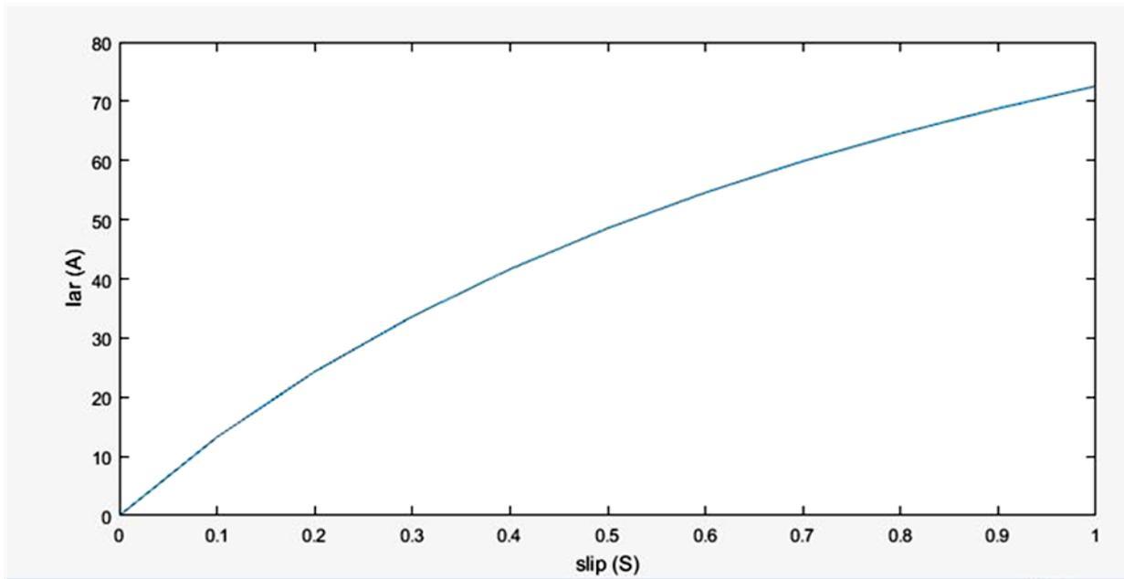
Fig 10: Rotor current against slip of 3-phase induction motor
