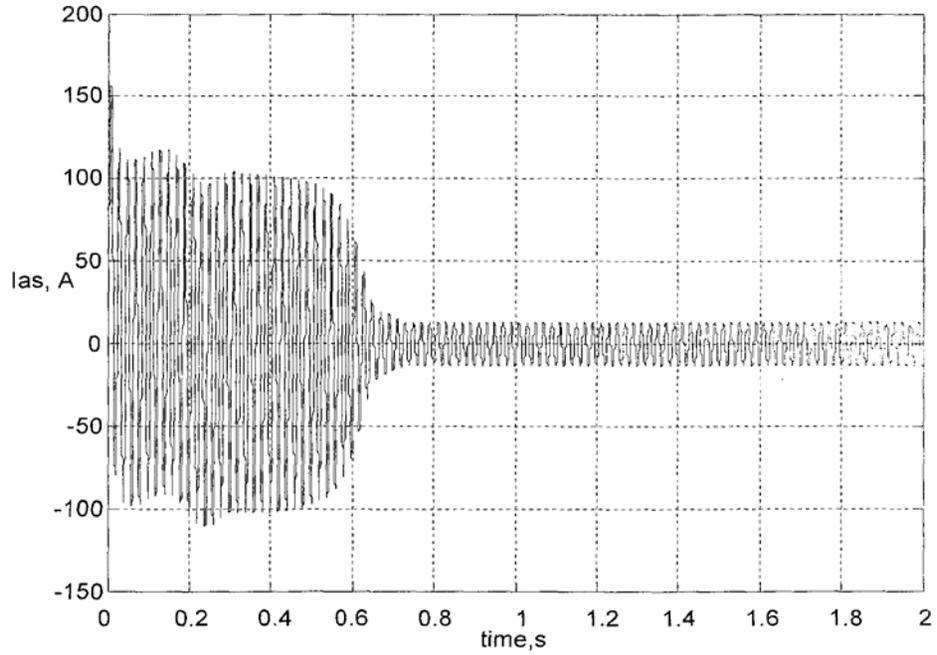
(a) Phase A Stator Current,  $I_{as}$
