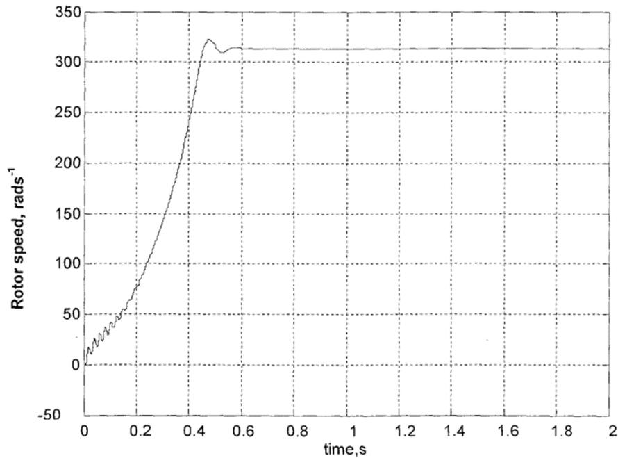
(b) At a torque load,  $T_L$ , of 3.5 N-m
