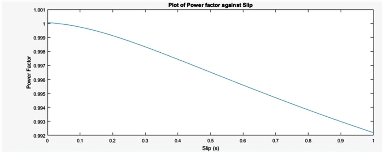
Fig 9 - Power factor/Slip characteristics of 3-phase induction motor
