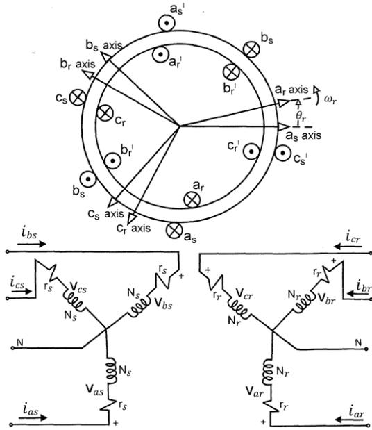
Fig 1: Two pole 3 – phase, star-connected symmetrical induction motor
