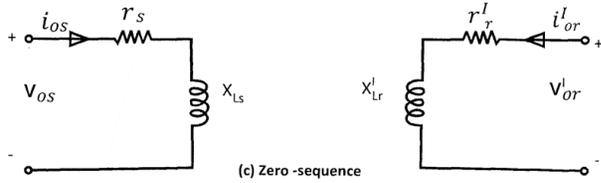
Fig 11: Dynamic equivalent circuit for 3-phase symmetrical induction machine in an arbitrary reference frame
