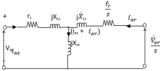
Fig 2: Per phase equivalent circuit of an induction motor
