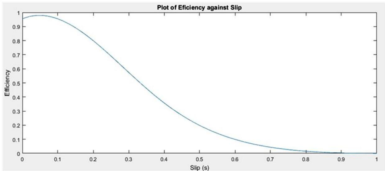
Fig 8 – Efficiency/Slip characteristics of 3-phase induction motor
