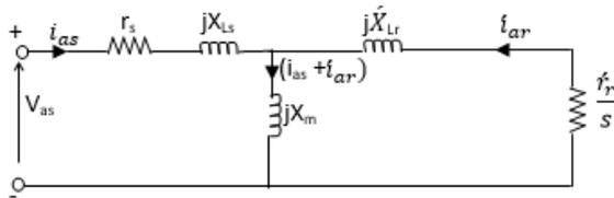
Fig 3: Per phase equivalent circuit of an induction motor at run condition with ( $s < 1$ ) and the rotor short circuited
