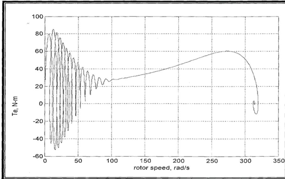
Fig 12 – The Electromagnetic Torque,  $T_e$  against rotor speed for the 3-phase induction machine (IM)
