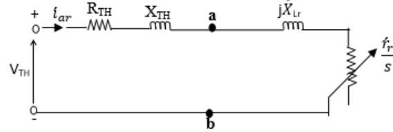
Fig 6: Thevenin equivalent of 3 – phase induction machine (motor) circuit model
