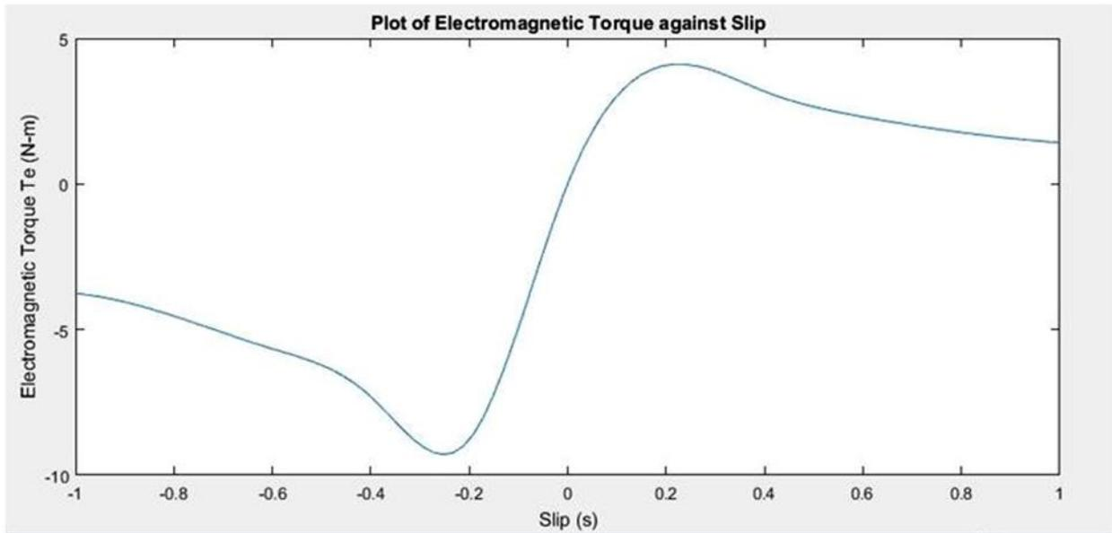
Fig 7: Torque/slip curve of a typical three –phase induction machine, operating at motoring/generating modes.
