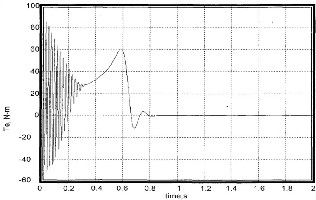
Fig 13 – The electromagnetic Torque,  $T_e$  against time for the 3-phase induction machine (IM)
