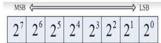
Figure b: Weighting of an 8- Bit Pixel
