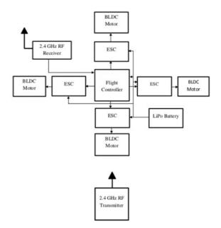
Fig: Drone architecture
