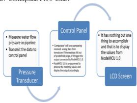
In case assume, there is a damage in the pipe, then the consequent transducer will obtain the pressure reading and it will transfer it to the comparator.
