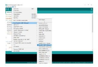
Since the NodeMCU 1.0 (ESP-12E Module) is a type of a arduino, hence we can directly burn the program over the ESP8266 using arduino IDE.
