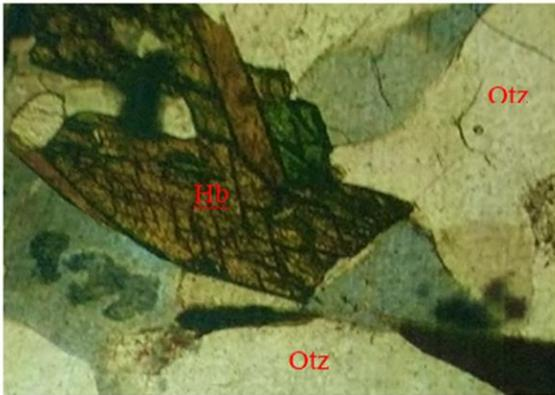
Figure 3: Photomicrograph of Granite Gneiss Showing Quartz (Qtz), and Hornblende (Hb).
