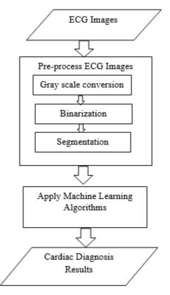
Fig. 1 The cardiac diagnosis system using ECG medical images
