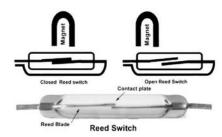
Figure 2: Operation Principle of Reed Switch
