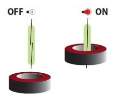
Figure 1: Configuration of Reed Switch
