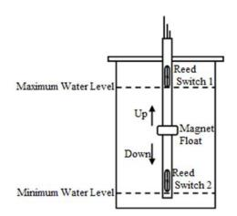
Figure 3.The assmble of tank with reed switch sensor A. The Sensor Mechanism
