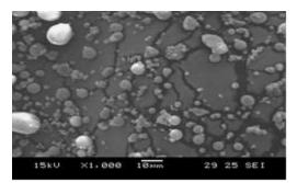
Fig. 1 SEM of Fly ash
