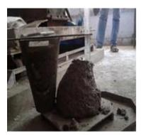
Figure 5 Measuring of Slump
