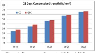
Figure 9 Compressive Strength of CC and GPC Cubes
