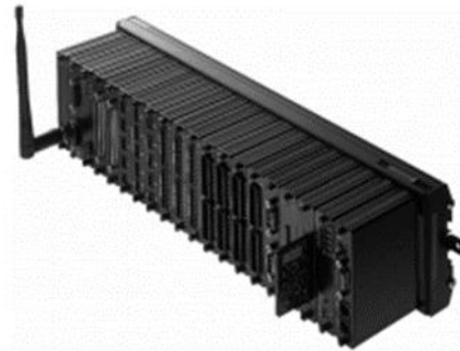
Figure 1 Example of a PLC: Festo IPC PS1 Professional
