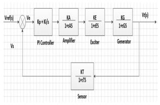
Fig. 1: Block diagram of the AVR system
