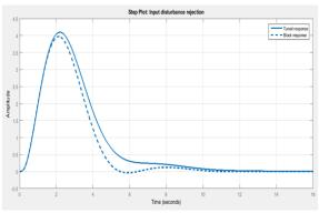
Fig. 11: Input disturbance rejection
