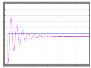
Fig. 5: Step Response for Non-compensated loop.
