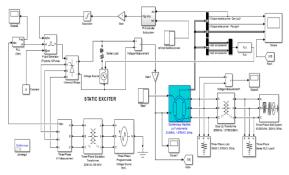
Fig. 4: SIMULINK Model for the Non-Linear Control loop
