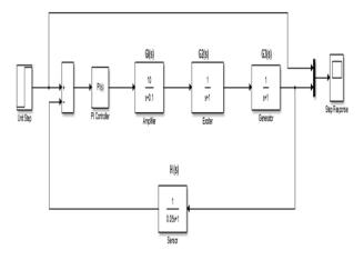
Fig. 2: SIMULINK Model of Transfer Functions
